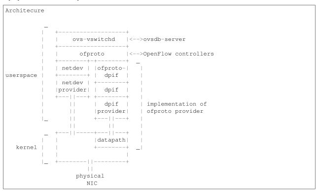
struct dpif\_class, in lib/dpif-provider.h, defines the interfaces required to implement a dpif provider for new hardware or software. That structure contains many function pointers, each of which has a comment that is meant to describe its behavior in detail. If the requirements are unclear, report this as a bug.
